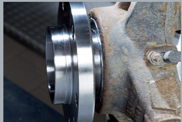
Image 3: The locking ring must lie flush with the steering swivel
